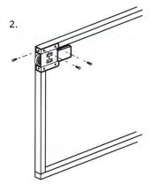
Lay door on edge & remove screws.
