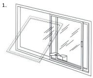
Open completely, lift up and out.
